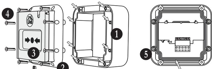
**Attention:** The o-ring sealant must be correctly fitted in the channel to provide the declared IP67 rating! /
