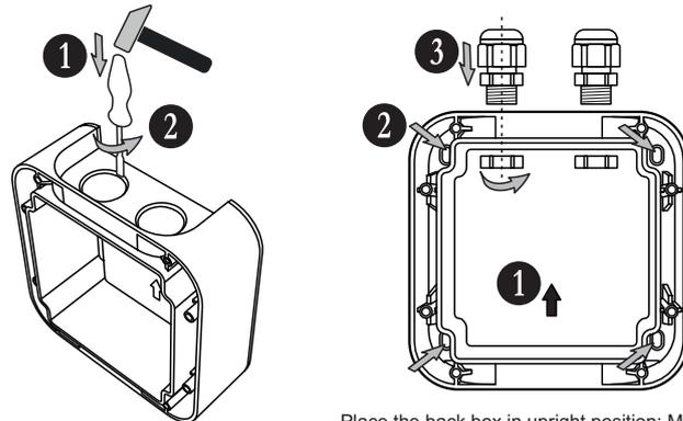
Remove the protective caps of the cable gland holes./
